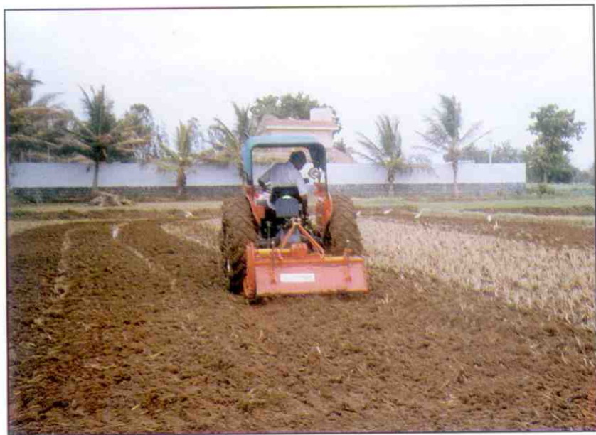
Fig 3 Field testing of Tractor mounted rotavator for seedbed preparation (dryland)
