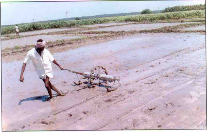
Fig 2 Field operation of low land rice seeder
