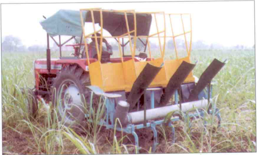
Fig.1 IISR Multipurpose planter in operation (Interculture mode)
