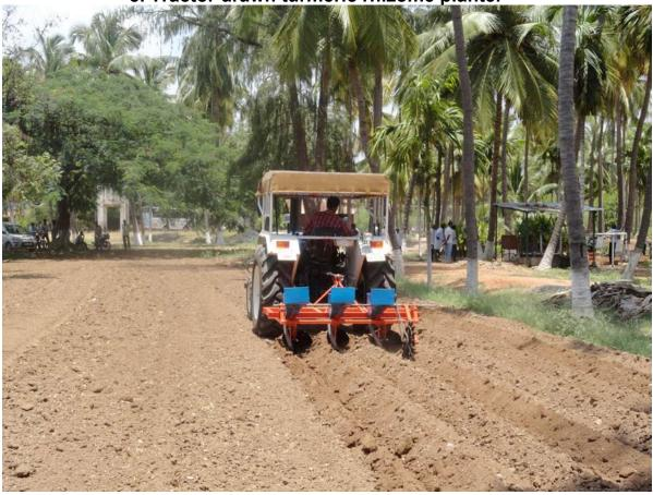
This unit can be operated by 35-45 hp tractor which has the facility to plant three rows at a time in the required spacing. Row spacing is adjustable and can cover 1.2 ha per day. Cost of the unit is Rs.50,000/-.
