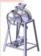
press the fruit gently against the rotor. The fruits are fed at the top manually. The fruits travel half the circumference and are dehusked in the process. The dehusked kernals fall to the bottom along with the husk. Tests were conducted with both the models. The speed was varied from 40 to 80 rpm. The results showed that the dehusking efficiency was 53 to 67%. The best dehusking performance was observed in 60 rpm. The breakage was observed in the range of 8 to 10 %.
