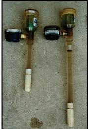
**Figure 1.** Experts recommend that producers take tensiometer readings at two depths.
