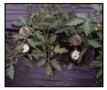
**Figure 12.** Two tensiometers set at two different depths give a good estimate of soil moisture at effective rooting and just below the root zone.
