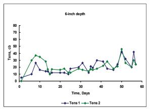
**Figure 15.** Comparison between two tensiometers set at a 6-inch depth at different crop locations within the tunnel.
