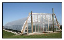
**Figure 1.** High tunnels are simple, plastic covered, passive-solar-heated structures.
