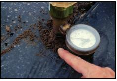
**Figure 5**. Firm the soil around the base of the tensiometer so that rain water does not run down the side of the tube and distort your reading.
