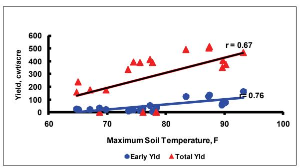
**Figure 4.** Polyethylene mulch effect on tomato yield as a result of 4-inch soil temperature, from 1997 to 2001 studies, lowa.
