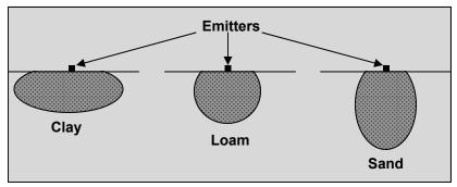
**Figure 10.** Soil wetting pattern from water application through a trickle system.
