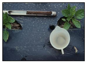
**Figure 4.** Add a small amount of water to the bottom of hole for good contact of ceramic cup to soil.
