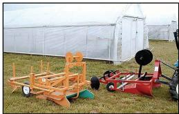
**Figure 8**. A "mini" mulch layer (right) is designed for high tunnel use.
