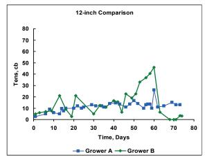
**Figure 14.** Two growers' ability to manage the deep tensiometer, 12 inch, at 10 cbar reading. A 10-cbar reading indicates aeration porosity and indicates ample water supply without excessive leaching or wide fluctuation in water quantity.
