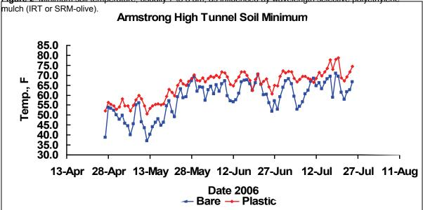
Figure 2. Minimum soil temperature, usually 7 to 8 am, as influenced by wavelength selective polyethylene.
