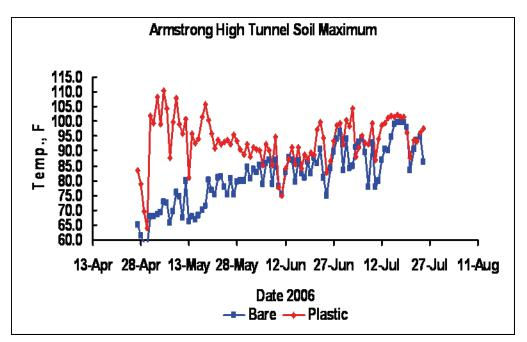
**Figure 3.** Effect of wavelength selective polyethylene mulch (ITR or SMR-olive) on the maximum soil temperature, usually 3 p.m.
