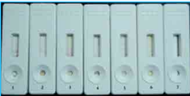
Lateral flow strip test for Classical swine fever virus antigen detection from TCF 1-6 positive TCF 7 - Negative TCF
